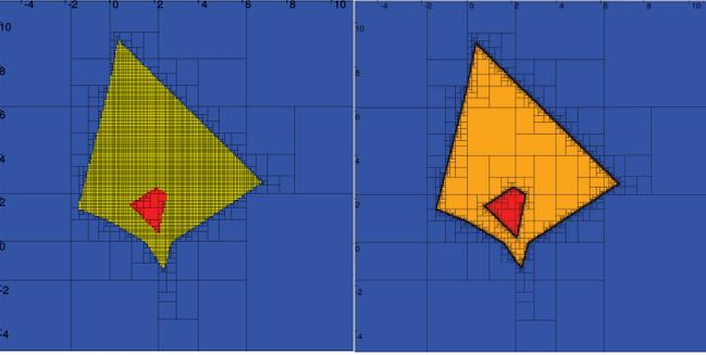
Fig. 2. Left: Classical interval methods accumulate on the yellow thick boundary (the penumbra). Right: the method we propose here allows a fast treatment of the penumbra. The frame box is  $[-5, 11]^2$
