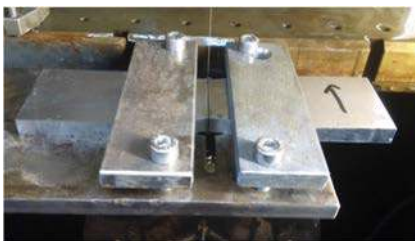
Fig. 16 Part clamping during wire electro-discharging machine cutting
