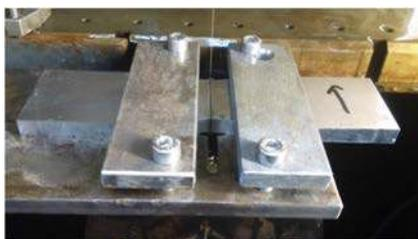
**Fig. 16** Part clamping during wire electro-discharge machine cutting
