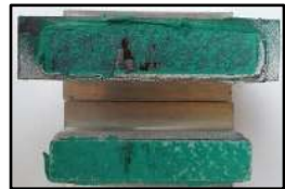
BM1822/Prepreg fracture for \gamma = 0^\circ
