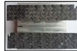
SP498/Prepreg fracture for \gamma = 0^\circ
