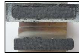
SP498/Prepreg fracture for \gamma = 45^\circ ; 90^\circ \text{ and } 135^\circ
