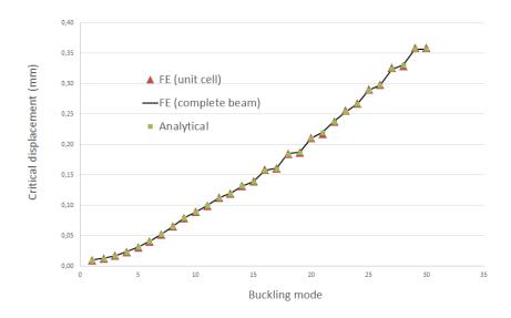
Figure 13: Comparison between the analytical and numerical critical displacements
