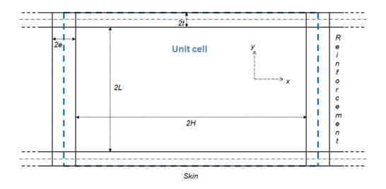
Figure 6: Unit cell model for the numerical modeling
