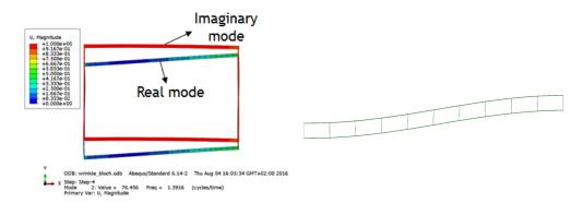
(a) Real and imaginary components of a unit cell (b) Corresponding rebuilt mode for the entire colmode umn
