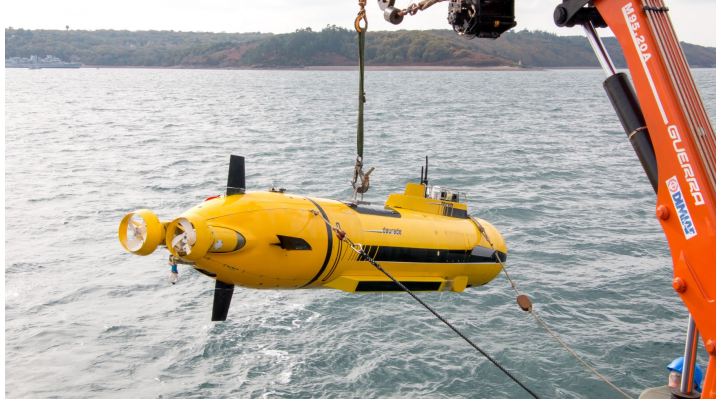
Figure 12: Daurade : the underwater robot used for our experiment. Photo: S. Rohou
