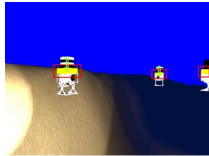
Fig. 9. Example of image processing for extraction of positions, sizes of robots and bar code. Red rectangle expresses the position and size of robot, green area is used for bar code decoding and getting the ID of robot.
