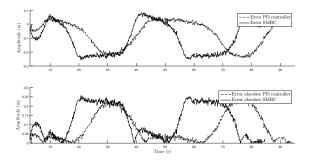
Fig. 8. Error comparison between PD controller and  ${\rm SMRC}$
