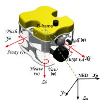
Fig. 1. B-frame and NED-frame of Underwater Vehicles
