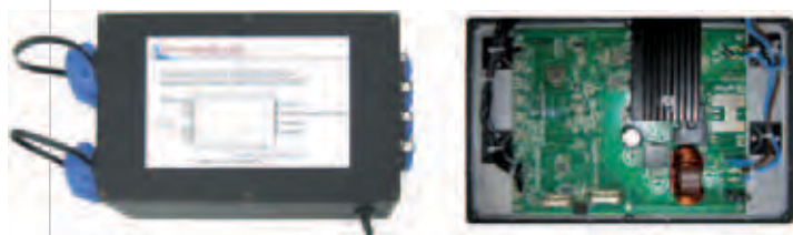
Figure 2: PSC of the Splashelec system in a waterproof case
