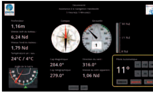
Figure 4: The human machine interface displays sensor information and contains a virtual keyboard (in yellow) to replace the physical one
