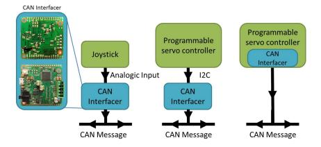
**Fig. 6** Examples of a CAN node: The joystick and the Programmable Servo Controller (PSC) in its first version. The next version will have a CANinterfacer integrated into the board.
