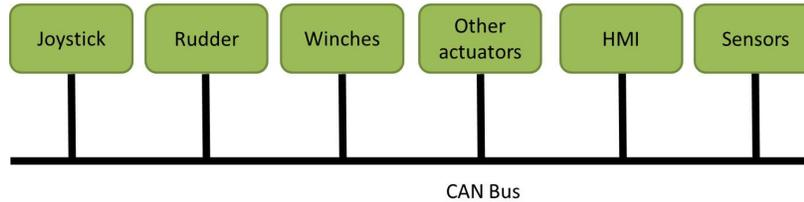
**Fig. 5** CAN architecture of the system
