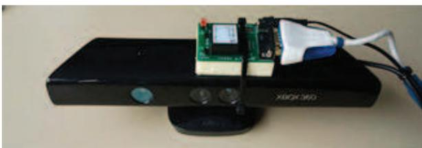
Figure 9. The IMU is fixed on the Kinect
