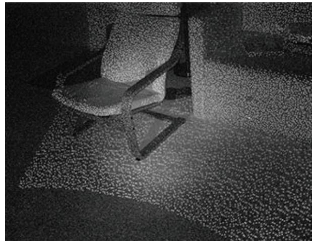
Figure 1. Kinect's projected IR structured light
