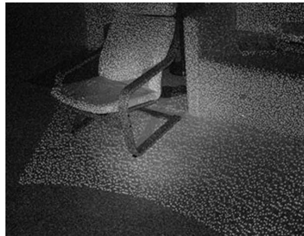
Figure 1. Kinect's projected IR structured light
