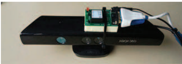
Figure 9. The IMU is fixed on the Kinect
