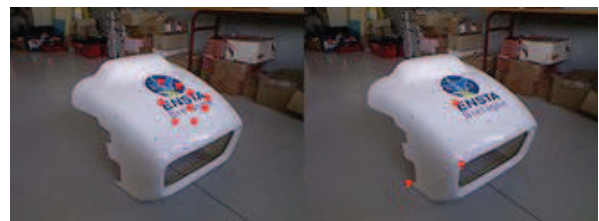
Figure 4. Selection of (a) 10 coplanar (b) 3 non-collinear correspondences
