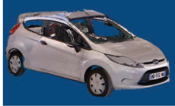
Figure 7. A car reconstructed from 7 kinect poses.
