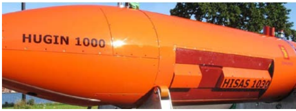
Fig. 2. The HISAS 1030 interferometric SAS mounted on a HUGIN autonomous underwater vehicle.
