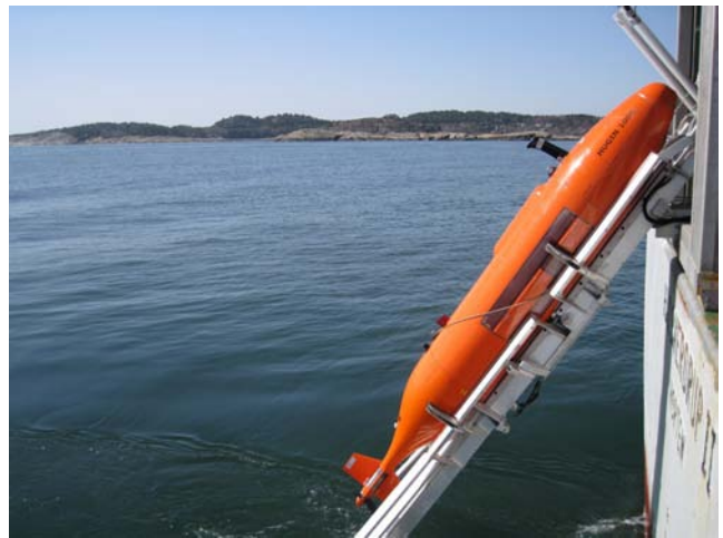
Fig. 1. The HUGIN HUS AUV during launch from H U Sverdrup II April 11, 2011.
